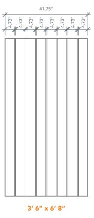
NOTE: BY REQUEST, DOOR HEIGHT COMES IN VARYING DIMENSIONS TO A MINIMUM OF 79". EXCESS WILL BE TAKEN FROM BOTTOM RAIL. ALL OTHER DIMENSIONS WILL REMAIN THE SAME.
