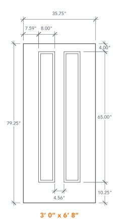
NOTE: BY REQUEST, DOOR HEIGHT COMES IN VARYING DIMENSIONS TO A MINIMUM OF 79". EXCESS WILL BE TAKEN FROM BOTTOM RAIL. ALL OTHER DIMENSIONS WILL REMAIN THE SAME.
