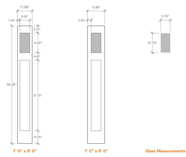
NOTE: BY REQUEST, SIDELITE HEIGHT COMES IN VARYING DIMENSIONS TO A MINIMUM OF 95". EXCESS WILL BE TAKEN FROM BOTTOM RAIL. ALL OTHER DIMENSIONS WILL REMAIN THE SAME.
