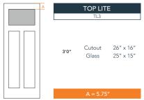
A = DISTANCE FROM TOP OF DOOR TO TOP OF OPENING. NOTE: PLASTPRO DOES NOT PROVIDE PRE-CUT CONFIGURATION SERVICE FOR THIS DOOR.
