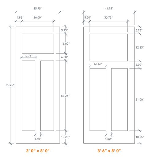
NOTE: BY REQUEST, DOOR HEIGHT COMES IN VARYING DIMENSIONS TO A MINIMUM OF 95". EXCESS WILL BE TAKEN FROM BOTTOM RAIL. ALL OTHER DIMENSIONS WILL REMAIN THE SAME.
