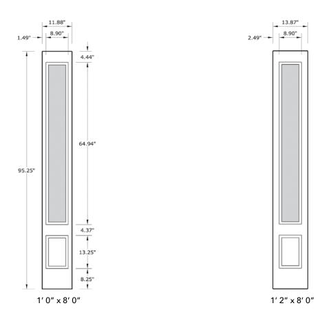
NOTE: BY REQUEST, SIDELITE HEIGHT COMES IN VARYING DIMENSIONS TO A MINIMUM OF 95". EXCESS WILL BE TAKEN FROM BOTTOM RAIL. ALL OTHER DIMENSIONS WILL REMAIN THE SAME.
