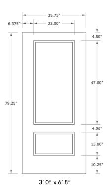
NOTE: BY REQUEST, DOOR HEIGHT COMES IN VARYING DIMENSIONS TO A MINIMUM OF  $79^{\circ\circ}$ . EXCESS WILL BE TAKEN FROM BOTTOM RAIL. ALL OTHER DIMENSIONS WILL REMAIN THE SAME.
