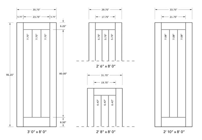
NOTE: BY REQUEST, DOOR HEIGHT COMES IN VARYING DIMENSIONS TO A MINIMUM OF 95". EXCESS WILL BE TAKEN FROM BOTTOM RAIL. ALL OTHER DIMENSIONS WILL REMAIN THE SAME.
