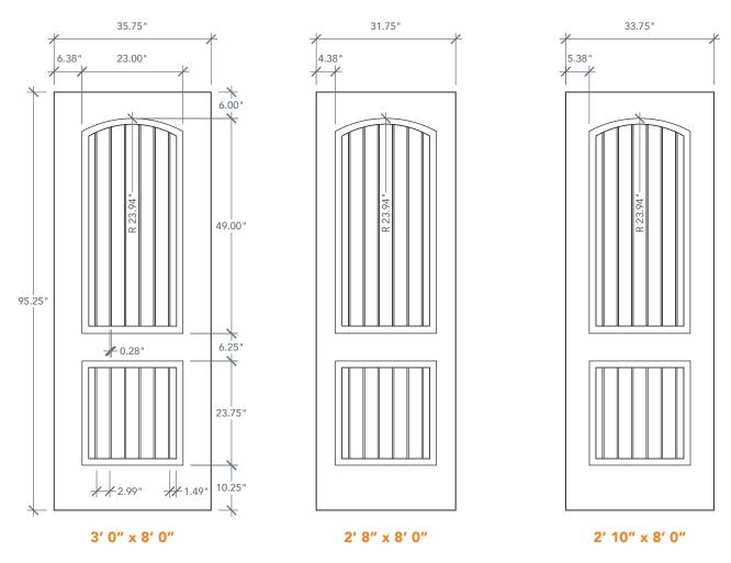
NOTE: BY REQUEST, DOOR HEIGHT COMES IN VARYING DIMENSIONS TO A MINIMUM OF 95". EXCESS WILL BE TAKEN FROM BOTTOM RAIL. ALL OTHER DIMENSIONS WILL REMAIN THE SAME.
