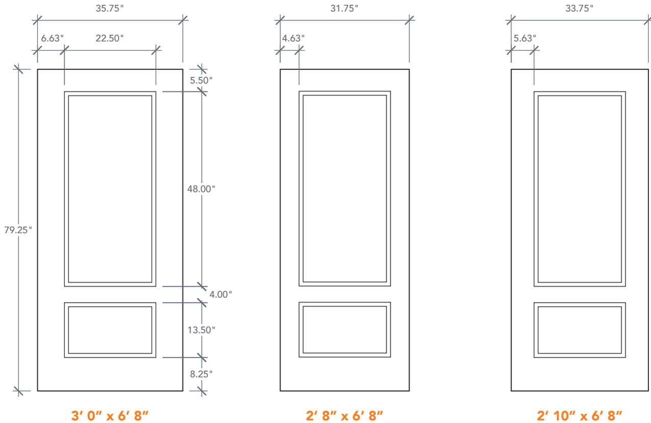
NOTE: BY REQUEST, DOOR HEIGHT COMES IN VARYING DIMENSIONS TO A MINIMUM OF 79". EXCESS WILL BE TAKEN FROM BOTTOM RAIL. ALL OTHER DIMENSIONS WILL REMAIN THE SAME.
