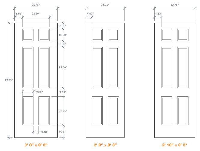
NOTE: BY REQUEST, DOOR HEIGHT COMES IN VARYING DIMENSIONS TO A MINIMUM OF 95", EXCESS WILL BE TAKEN FROM BOTTOM RAIL. ALL OTHER DIMENSIONS WILL REMAIN THE SAME.
