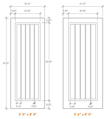
NOTE: BY REQUEST, DOOR HEIGHT COMES IN VARYING DIMENSIONS TO A MINIMUM OF 95". EXCESS WILL BE TAKEN FROM BOTTOM RAIL. ALL OTHER DIMENSIONS WILL REMAIN THE SAME.
