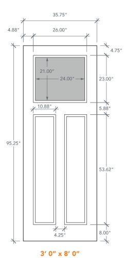
NOTE: BY REQUEST, DOOR HEIGHT COMES IN VARYING DIMENSIONS TO A MINIMUM OF 95". EXCESS WILL BE TAKEN FROM BOTTOM RAIL. ALL OTHER DIMENSIONS WILL REMAIN THE SAME.
