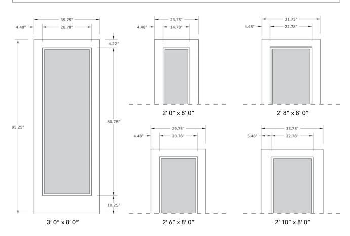
NOTE: BY REQUEST, DOOR HEIGHT COMES IN VARYING DIMENSIONS TO A MINIMUM OF 95". EXCESS WILL BE TAKEN FROM BOTTOM RAIL. ALL OTHER DIMENSIONS WILL REMAIN THE SAME.
