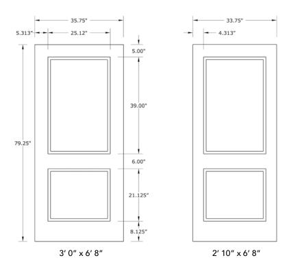
NOTE: BY REQUEST, DOOR HEIGHT COMES IN VARYING DIMENSIONS TO A MINIMUM OF  $79^{\circ\circ}$ . EXCESS WILL BE TAKEN FROM BOTTOM RAIL. ALL OTHER DIMENSIONS WILL REMAIN THE SAME.
