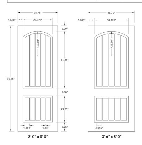
NOTE: BY REQUEST, DOOR HEIGHT COMES IN VARYING DIMENSIONS TO A MINIMUM OF 95". EXCESS WILL BE TAKEN FROM BOTTOM RAIL. ALL OTHER DIMENSIONS WILL REMAIN THE SAME.
