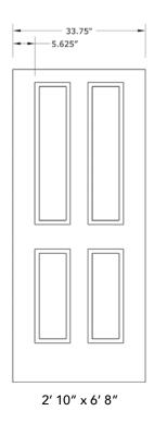
NOTE: BY REQUEST, DOOR HEIGHT COMES IN VARYING DIMENSIONS TO A MINIMUM OF 79". EXCESS WILL BE TAKEN FROM BOTTOM RAIL. ALL OTHER DIMENSIONS WILL REMAIN THE SAME.
